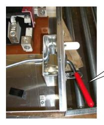
Put the handle crank into the lower position.
