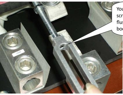
You must start with the top turnbuckle screw (attached to the switch movable) flush with the inside of the turnbuckle body.
